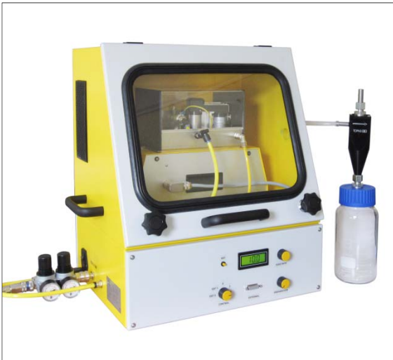
Dust Generator Unit (DGU 413) with SAG 410 U and cyclone
