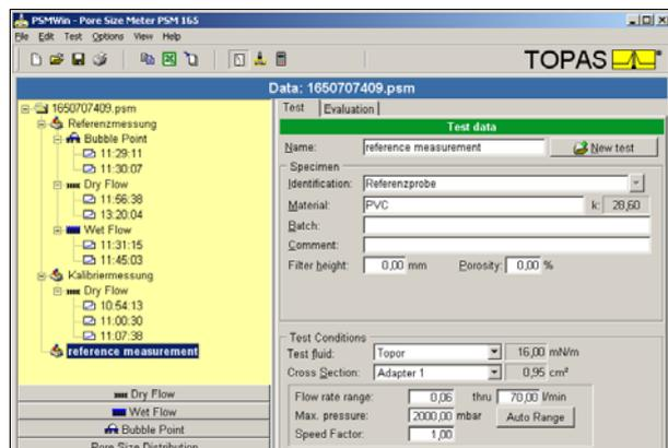
Input dialog for sample data and test conditions
