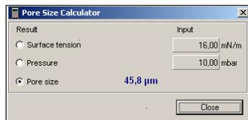
Pore size calculator for evaluation of the measuring range
