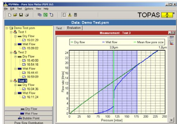
Measuring data window with a dry flow curve (green) and a wet flow curve (blue); light blue colored background: analyzed pressure range
