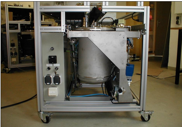
ATM243 (with pressure-proof housing) in the Test Rig SPT 140
