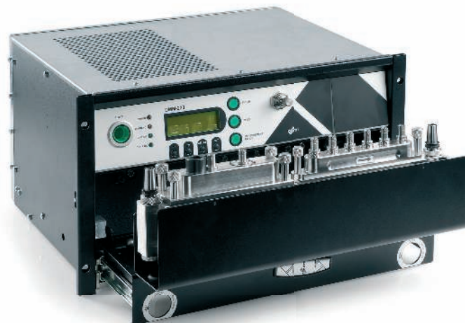
Dekati® Mass Monitor with impactor hatch opened
